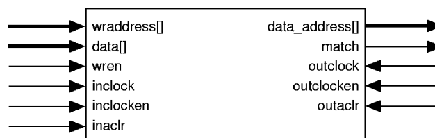
Figure 22. APEX 20KE CAM Block Diagram
